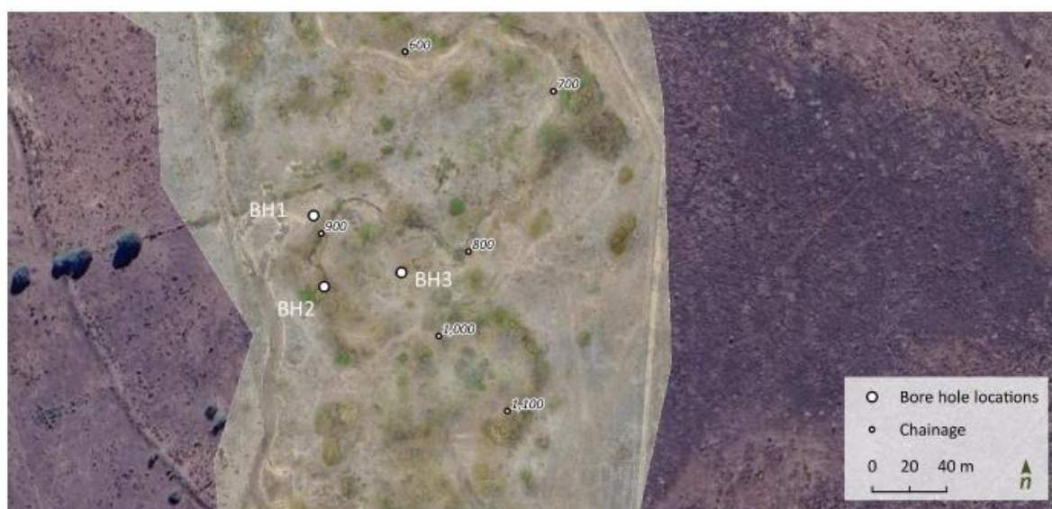
Figure 12. Geotechnical investigation borehole locations at the Kroombit Creek tributary site
